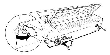
3. If your cable has a ground wire, attach it to the ground connector beneath the interface connector.
